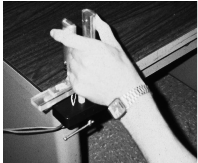
Figure 1. Testing apparatus for measuring the isometric gripping strength of the thumb and index finger.
