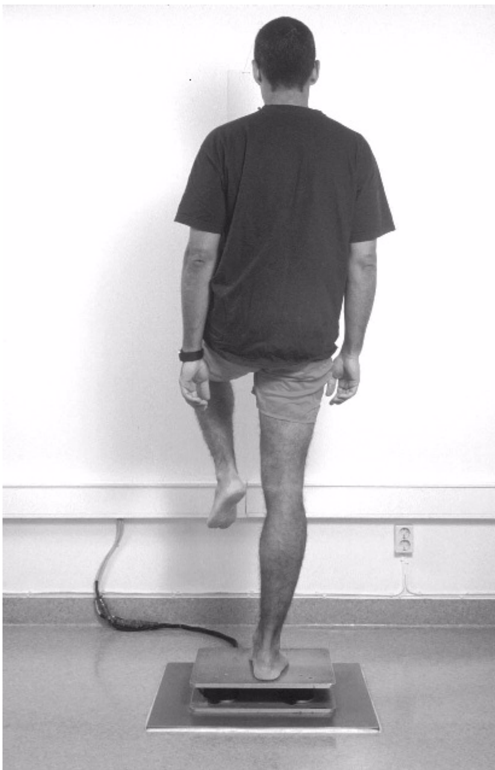
Figure 1 Stabilometry in single-limb stance, tested by means of a strain gauge force plate. A standardized position was used. The subject is a model who did not participate in the study.
