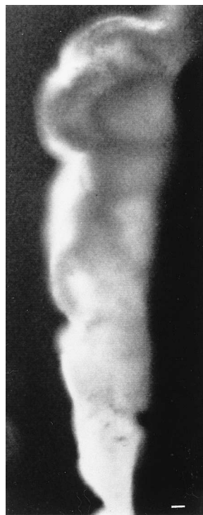
FIG. 10. Nonconfocal laser scanning dark field photomicrograph of a 77-day-old bacterial GAC-coated particle showing variation of the biofilm thickness on the same colonized surface. Bar, 15 \mu\text{m} .
