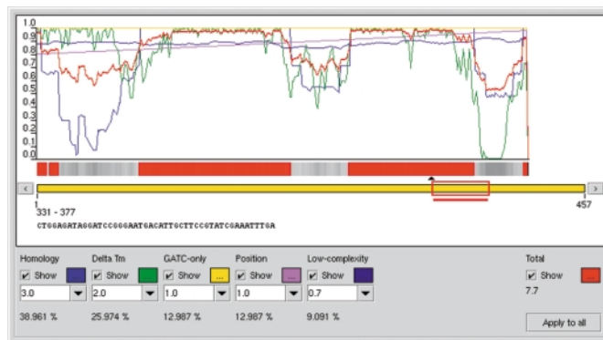
Figure 1. Screenshot of part of OligoWiz's graphical interface. The graphs demonstrate the score of oligonucleotides along the length of the transcript sequence. The red graph (total) represents the total weighted score from which the automated oligonucleotide selection is based. The red box placed on the orange bar is a handle for manual oligonucleotide selection. Below the graphs the weights for the parameter scores can be set. Shown is the S.cerevisiae transcript AA417464.
