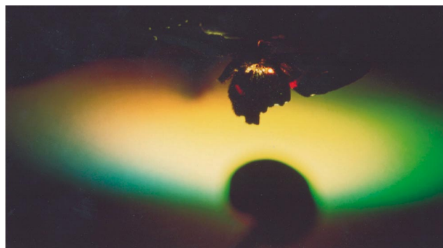
Figure 2. Real-colour photograph illustrating the range of hues produced from a single iridescent region of wing (region A from the inset picture in figure 1 a ). A narrow beam of collimated white light, incident normally on iridescent region A, produces this very broad range of colour, each one reflected at a slightly different angle.
