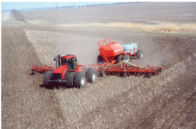
Fig. 1. Seeder (drill) designed to simultaneously seed and fertilize corn, wheat, soybeans, canola, or other agronomic crop directly (no-till) into undisturbed soil and residue of the previous crop left lying on the soil surface. This drill, developed by Horsch Equipment Manufacturing (Schwandroft, Germany) and in use on the private farm of Agro Soyus in South Central Ukraine near Dnepropetrovsk, is 18 m wide and can plant at speeds up to 16 km/hr (nearly 30 hectares/hr), not including time required to refill the seed and fertilizer tanks. The tools (openers) used on this drill to place seed at one level, e.g., 3 cm deep, and fertilizer beneath the seed, e.g., 7–8 cm deep, are spaced 30–40 cm apart, depending on the crop and yield potential of the region; these tools were developed by Anderson Machine (Andover, SD).
