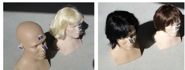
Fig. 1 Measurement of solar ultraviolet radiation on ears in relation to hair cover using head-forms and polysulfone dosimeters
