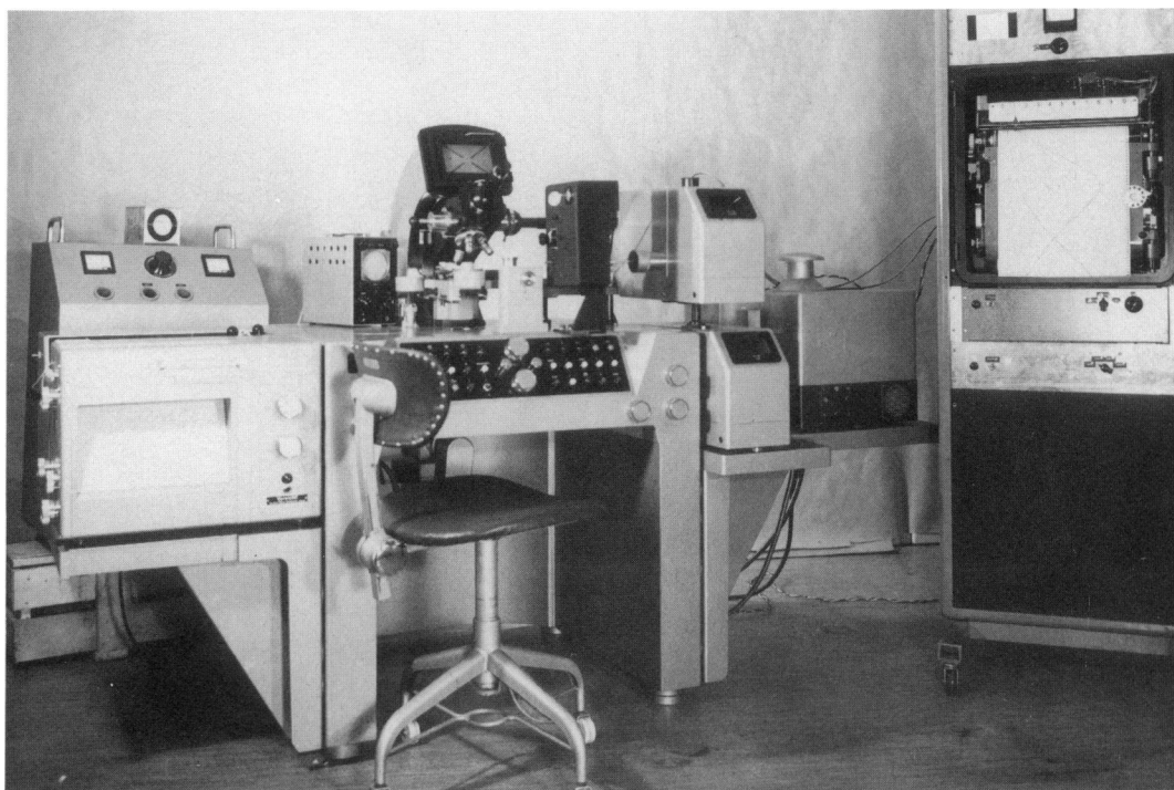
Figure 5 Recording, scanning high-resolution microspectrophotometer for UV and visible spectral regions (230–700 nm)
