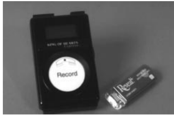
Figure 2 Cardiac event monitoring allows the recording of an ECG during symptoms. Non-invasive monitors such as the King of Hearts can be worn for weeks or even months at a time. The implantable Reveal monitor (Medtronic Inc.) is useful where monitoring is required for a prolonged period of time or where compliance is poor. It is easily implanted in a small subcutaneous pocket and allows monitoring for up to 14 months.
