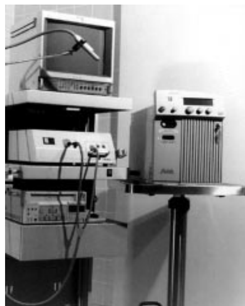
Figure 2 Whole endoscopy system consisting of light source, video recorder, and video screen.
