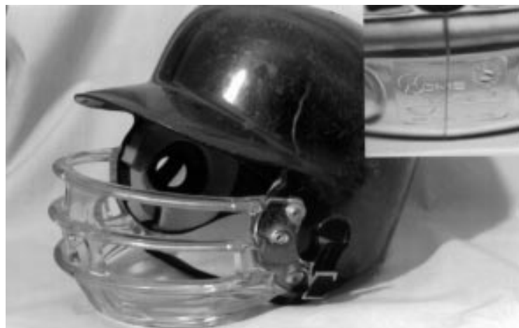
Figure 1 A baseball face guard consisting of a polycarbonate arch affixed to the ear flaps of a standard batter's helmet. Inset: close up photograph of a fracture in the arch caused by a pitched ball impact while worn by an 8 year old face guard team batter. This product was manufactured to the specifications of ASTM F910, which prevents facial contact from a baseball fired at 69 miles per hour. 10 11
