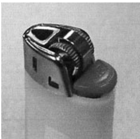
Figure 1 Cigarette lighter with a child resistant ignition mechanism. Note: This is one of many types of child resistant mechanisms. The metal shield must be depressed before the sparkwheel can be turned to produce a spark. The force required to depress the shield is difficult for young children to achieve.
