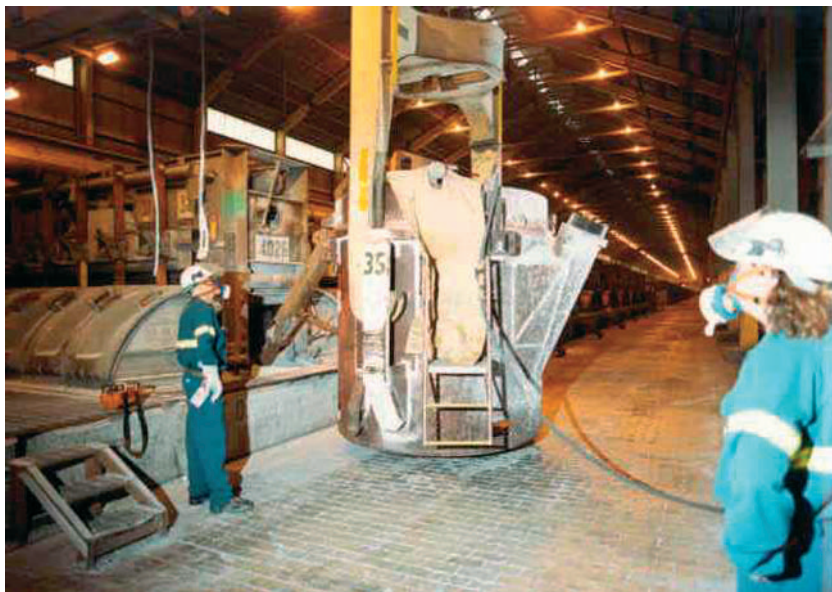
Figure 2 Potroom workers tapping metal in the pre-bake potroom.
