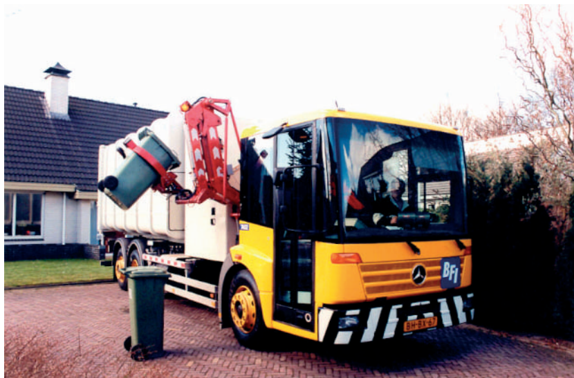
Figure 4 An example of a refuse truck with an automatic side collection system.
