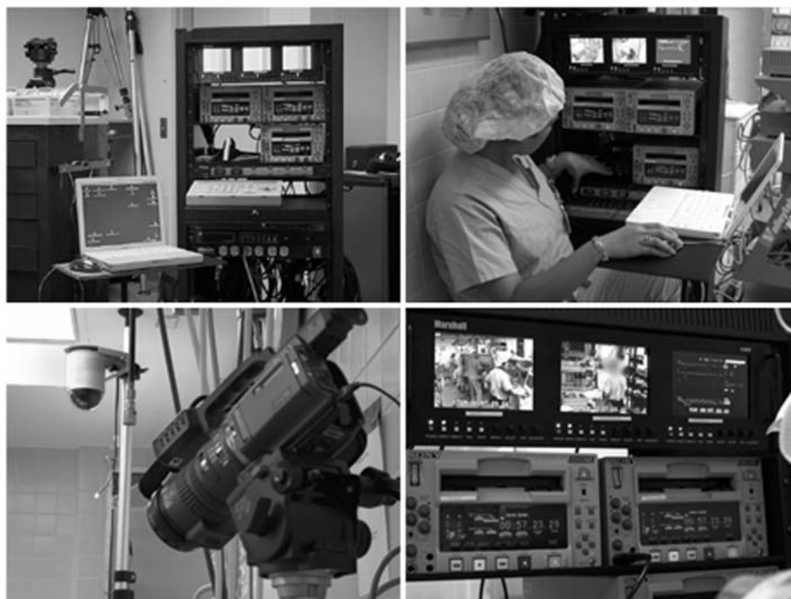
Figure 1 Clinical data collection system. Four views of our current data collection cart and associated video cameras. The data collection system includes three digital videotape recorders, two cameras, wireless and wired audio recording, time code synchronization, and a laptop computer running custom software for behavioral task analysis and clinical workload assessment.
