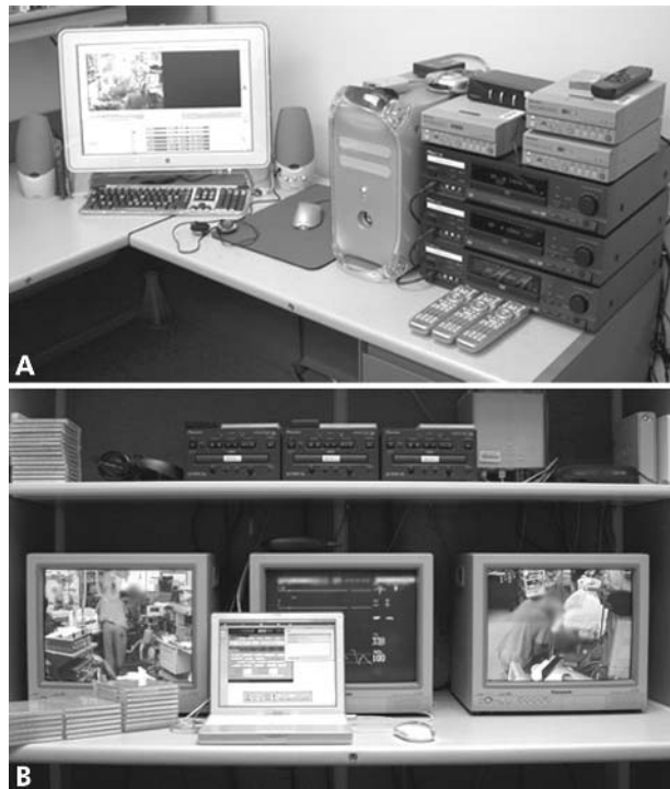
Figure 3 Digital video processing, archiving, and viewing stations. (A) DVD creation station (right) where three digital videotapes containing raw clinical video footage are burned directly to MPEG-2 encoded video on DVD. To the left is the non-linear digital video editing station, an Apple Macintosh dual processor G4 computer running commercially available software. (B) DVD review station. A computer running custom software controls three industrial grade DVD players attached to high quality color monitors. The review software permits synchronized playback of any case segment and annotative text entry (with associated case time) linked to our clinical event database.
