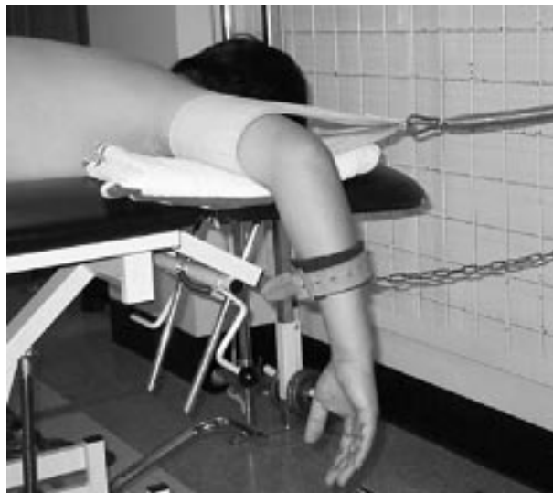
Figure 1 Each subject was positioned on a plinth in the prone position as in the standard internal rotation muscle test. A leather wrist strap was positioned 15 cm distal to the olecranon process and, via a chain, was securely attached to a strain gauge. To avoid glenohumeral adduction during the testing procedure, the humerus was stabilised using a sling attached to a grid in front.
