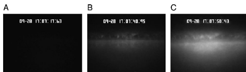
Figure 6. (A – C) Fluorescence microscopy images illustrating the buildup of fluorescent material from targeted nanodroplets along the wall of a 200- \mu\text{m} vessel due to US.
