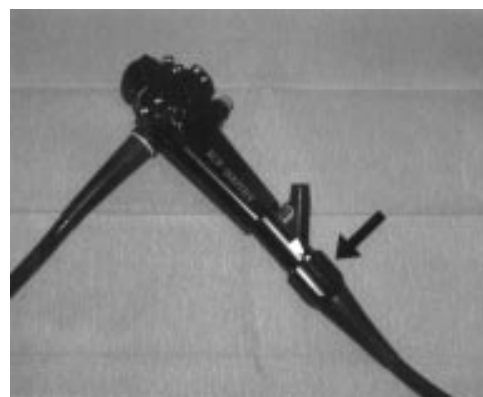
Figure 1 The control head of the variable stiffness colonoscope (Olympus XCF-SH230L). The dial for controlling the stiffness is arrowed. Specifications: distal end outer diameter 13.6 mm, flexible tube outer diameter 12.9 mm, instrument channel 3.2 mm, and working length 168 cm.
