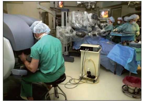
Fig 3 The da Vinci surgical system, which allows the surgeon to do laparoscopic surgery using robotic arms while looking at a three dimensional image from cameras inserted into the patient
