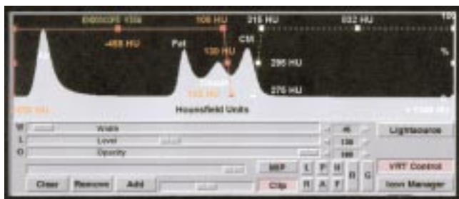
Figure 1 Volume rendering controls with a histogram showing voxel density values. The x axis shows the voxel values, the y axis the frequency distribution. The first peak represents air, the second fat, the third tissue, and the fourth contrast medium (CM). The orange graph represents the range used for visualising vessel, the white graph represents the range used for visualising calcification.
