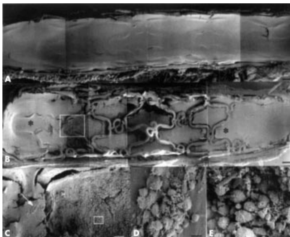
Figure 2 Low power scanning electron micrograph of control stent (A) and 48 \mu Ci stent (B) at 12 months. The entire control stent is endothelialised, whereas the 48 \mu Ci stent is endothelialised at the ends (* in B). Parts of the central portion of the 48 \mu Ci stent are non-endothelialised, and bare or partially covered struts are present. The transition zone between endothelialisation and non-endothelialisation is outlined in B and shown at medium power in C. Two areas are further magnified (arrow and box in C corresponding to D and E, respectively) to show adherent platelets and inflammatory cells on partially endothelialised (D) and non-endothelialised (E) parts of the stent. Bars = 0.5 mm in A and B, 0.1 mm in C, 0.01 mm in D and E. Reproduced from: Farb A, et al. Circulation 2001; 103 :1912–9, with permission of the American Heart Association.
