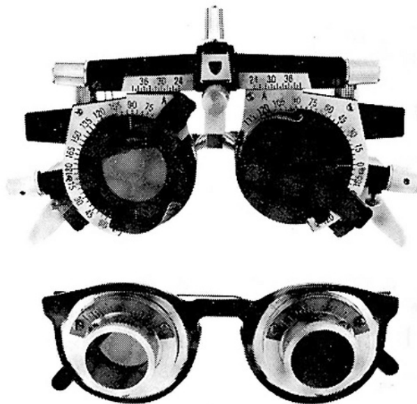
Figure 2 Threshold Amsler grid lenses containing pairs of polarised filters in each ocular. As the front filter is rotated, light transmission is reduced.
