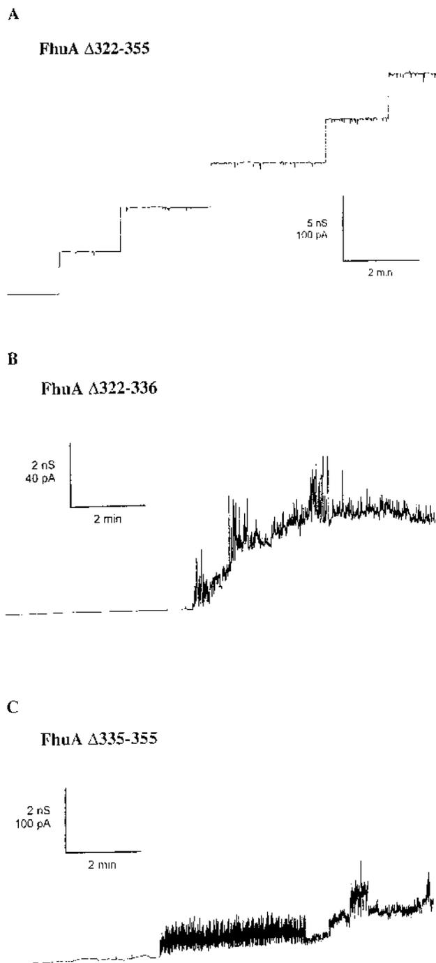
FIG. 5. Single-channel conductance of a diphytanoyl phosphatidylcholine membrane separating two aqueous compartments containing 0.1 M KCl (A) or 1 M KCl (B and C) to which was added 5 ng of FhuA  $\Delta$ 322-355 (A), FhuA  $\Delta$ 322-336 (B), or FhuA  $\Delta$ 335-355 (C) per ml. The membrane voltages were 20 mV (A and B) and 50 mV (C).
