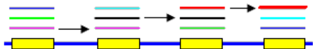
Figure 4 A chain of hits meeting CRISPR criteria. CRISPR arrays are identified by following chains of hits. Starting with a given pile, each hit that connects this pile to another pile later in the genome is a potential link in the chain. All possible chains are explored, abandoning the search each time the chain violates the criteria used for CRISPR array recognition (see Table 2). These criteria include maximum and minimum repeat length, maximum and minimum spacer length, and measures of the variance in repeat and spacer lengths. Shorter links are explored before longer links as regularly spaced arrays will be obtained by skipping every second, third... repeat. The figure shows the correct chain (arrows) for the example array from Fig. 3.
