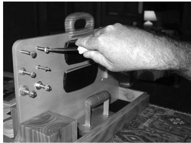
Figure 1 Photograph of a patient undertaking one of the tasks in the Sollerman grip function test, showing his ability to use a screwdriver to turn a screw into the board.
