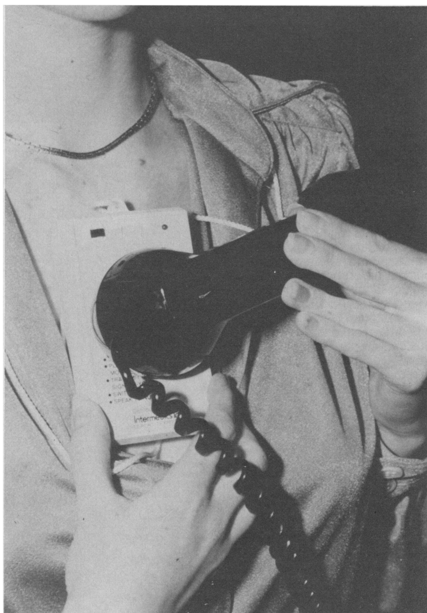
FIG. 1—Transtelephone transmitter of electrocardiographic signals placed against upper part of chest; mouthpiece of telephone receiver placed against transmitter.
