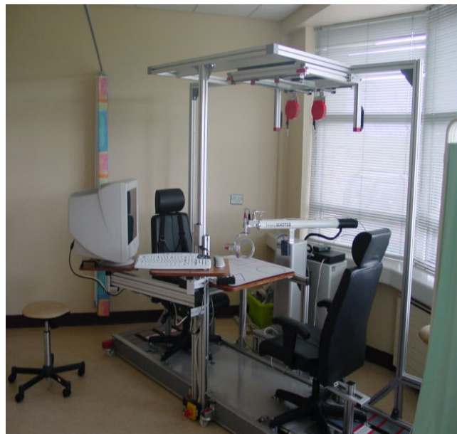
Figure 1 The GENTLE/S system as used in the clinical trial. The clinical prototype resulting from brainstorming with patients, clinicians, healthcare professionals and industrial parties.
