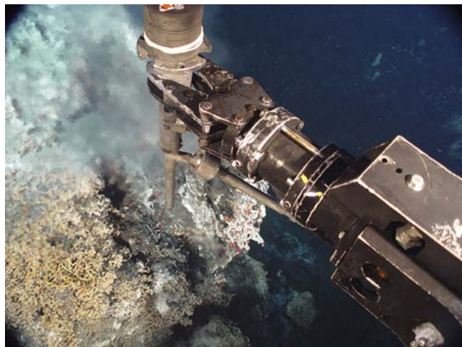
Figure 2. A Remotely Operated Platform Samples Vent Fluids from the Northeast Pacific Ocean
