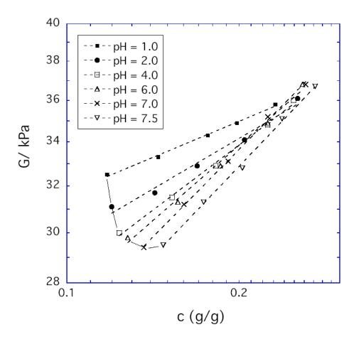
1. Elastic shear modulus as a function of polymer weight fraction for HPMA/DMA/TEGDMA hydrogels (70/30/02 mole ratio) at the pH values given in the legend and at fixed environmental NaCl concentration (0.15 M).
