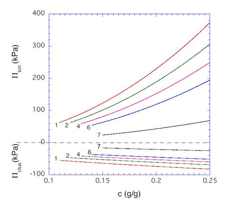
**3.** Estimated value of the counterion contribution to the osmotic swelling pressure, and of the contribution of microclusters to the swelling pressure, as a function of polymer concentration in the HPMA/DMA/TEGDMA hydrogels (70/30/02 mole ratio) at various pH values.
