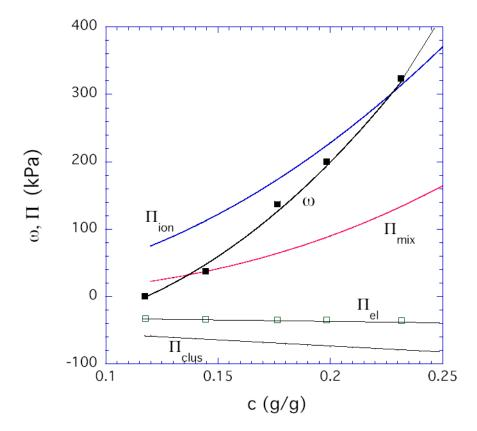
4. At pH = 1, the concentration dependence of the four contributions to the osmotic swelling pressure for the HPMA/DMA/TEGDMA hydrogels (70/30/02 mole ratio).
