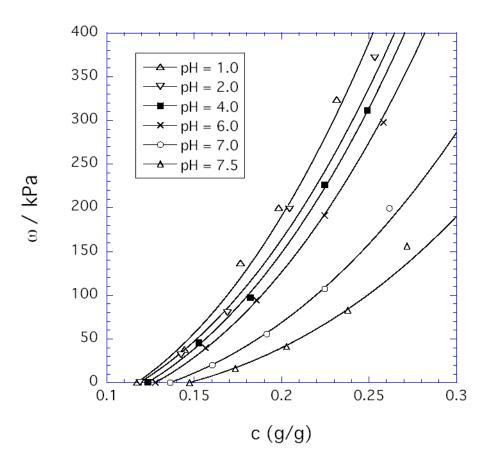
**2.** Osmotic swelling pressure as a function of polymer weight fraction in the HPMA/DMA/ TEGDMA hydrogels (70/30/02 mole ratio) at the pH values given in the legend and at fixed environmental NaCl concentration (0.15 M). The solid curves were obtained by least squares fit to a scaling equation (Equation 1).
