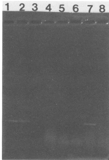
FIG. 3. Sensitivity of amplification of Tn5 sequences from Pima clay loam: detection by agarose gel electrophoresis. Lanes: 1, 3 \times 10^8 CFU; 2, 3 \times 10^7 CFU; 3, 3 \times 10^6 CFU; 4, 3 \times 10^5 CFU; 5, 3 \times 10^4 CFU; 6, 3 \times 10^3 CFU; 7, positive control (UAZ 302::Tn5 DNA); 8, uninoculated soil.
