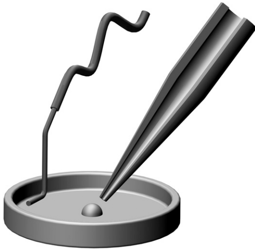
FIGURE 3 Schematic representation of single-cell electroporation geometry. The pulled end of the capillary is close to the targeted cell and is positioned at \sim 45^\circ with respect to the dish normal. The full capillary is much longer than shown. Its distal end is placed in a vial of buffer where an electrode that delivers electrical pulse is found. The capillary is filled with the same conducting buffer (not illustrated) that surrounds the cell. The electrical circuit is completed with a ground electrode placed far away from the targeted cell.
