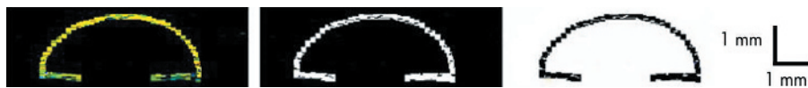
Figure 2 The cross sectioned images of the OCT scanning after calibration in mm were processed with the manufacturer's software. The pseudo-colours (left) were changed to black and white (middle) and then inverted (right) before fitting a polynomial equation in order to calculate the arc length.
