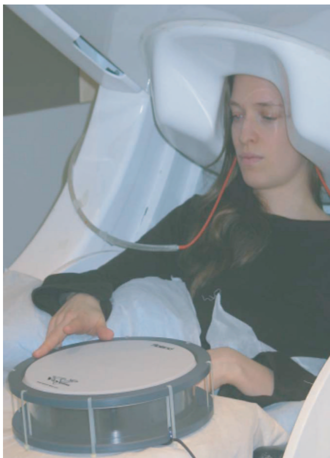
Fig. 1. Experimental setup. The subject, sitting with her head supported by the helmet-shaped neuromagnetometer, is tapping the nonmagnetic drum with her right index finger while looking at her hand.
