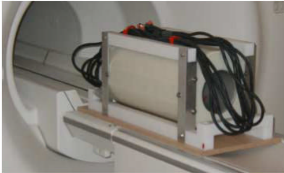
Figure 1. High-strength insert gradient coil on the patient table of a clinical 3T human scanner.
