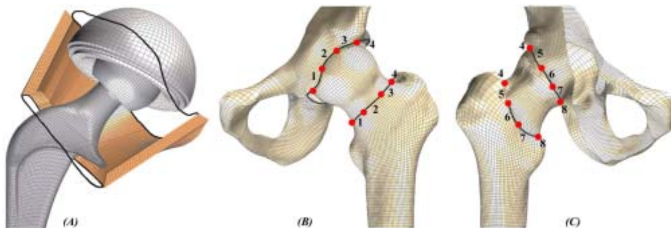
Figure 1. (A) Cut-away of the bony members, illustrating the finite element mesh of THA components and the capsule representation. The dark black lines illustrate the anatomic capsule attachment locus. (B) Anterior and (C) posterior views of the hemi-pelvis and femur finite element mesh, where the individual capsule sector definitions are identified by the red dots.
