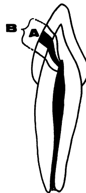
Fig 2 Diagrammatic representation of the path taken by an electric current through a human tooth. A represents a small electrode area. B represents a large electrode area
