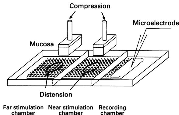
**Figure 1** Diagram of the divided organ bath used for recording motility reflexes in segments of isolated ileum. Distension or mucosal compression stimuli were applied in the near or far stimulation chambers, and the reflex responses of the circular muscle were monitored in the recording chamber. Each chamber was independently perfused and partitions (15 mm apart) prevented fluid mixing between chambers.
