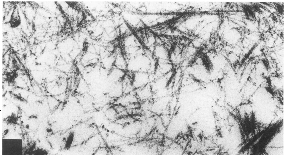
Figure 5 —Loosely arranged fibrillar material present in some lumens. (x 100,000)
