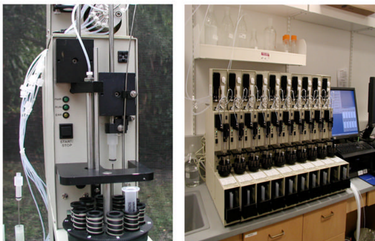
Figure 1. RapidTrace SPE workstation. (left, single modular unit for 10 cartridges; right, ten units controlled by a PC)
