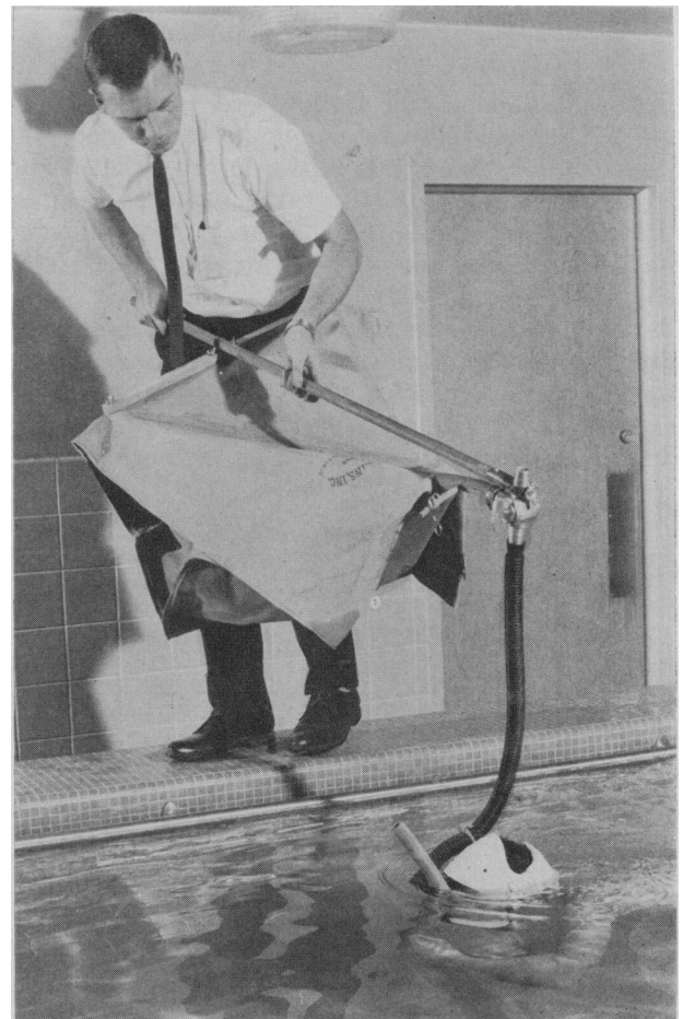
Fig. 3.—Air collection in Douglas bag during swimming.
