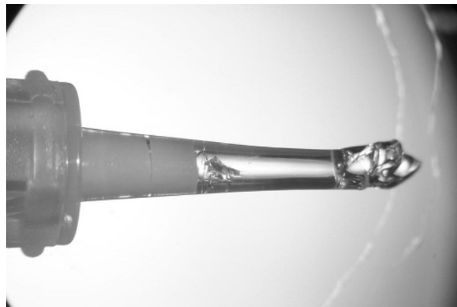
Figure 3 Gross photograph of the injection process of the C-flex intraocular lens (IOL) through the R-INJ-04 soft-tipped injector. The plunger is manufactured from a soft material. This allows it to compress during the progression through the narrowing nozzle and by doing that the plunger fills the nozzle completely and tightly. Thus, if loaded correctly, no part of the lens can be trapped between the plunger and the nozzle, and also over-ride of the plunger over the IOL is impossible.
