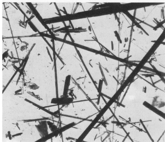
Figure 1 Transmission electron micrographs of: (a) standard UICC crocidolite - inoculum; (b) standard UICC crocidolite - recovered from granuloma of animal without mesothelioma; (c) standard UICC crocidolite - recovered from granuloma of animal with mesothelioma; (d) 2 h milled crocidolite - inoculum; (e) 2 h milled crocidolite - recovered from granuloma of animal without mesothelioma; (f) 2 h milled crocidolite - recovered from granuloma of animal with mesothelioma.
