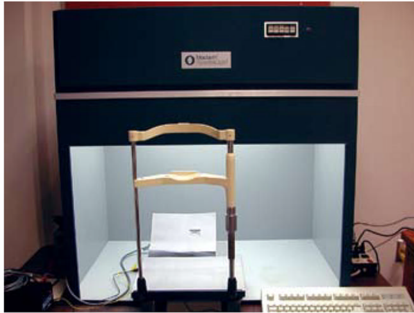
Figure 2. Porcelain color discrimination test apparatus, which includes optometrist's frame/chin rest, porcelain color discrimination test wheel within Macbeth SpectraLight Booth, and computer keyboard used by subjects next to booth.
