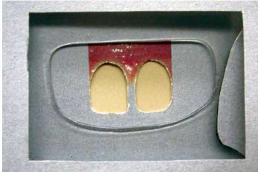
Figure 1. Porcelain color discrimination test wheel cover with edge of open shutter visible toward right. Pair shown has negligible color difference.
