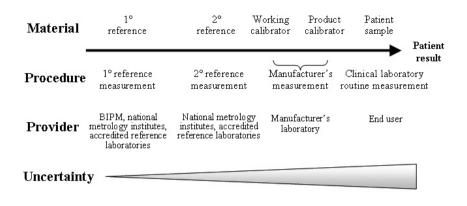
Figure. A generic calibrator traceability flowchart. Based on ISO 17511:2003 Fig 4.2.2.
