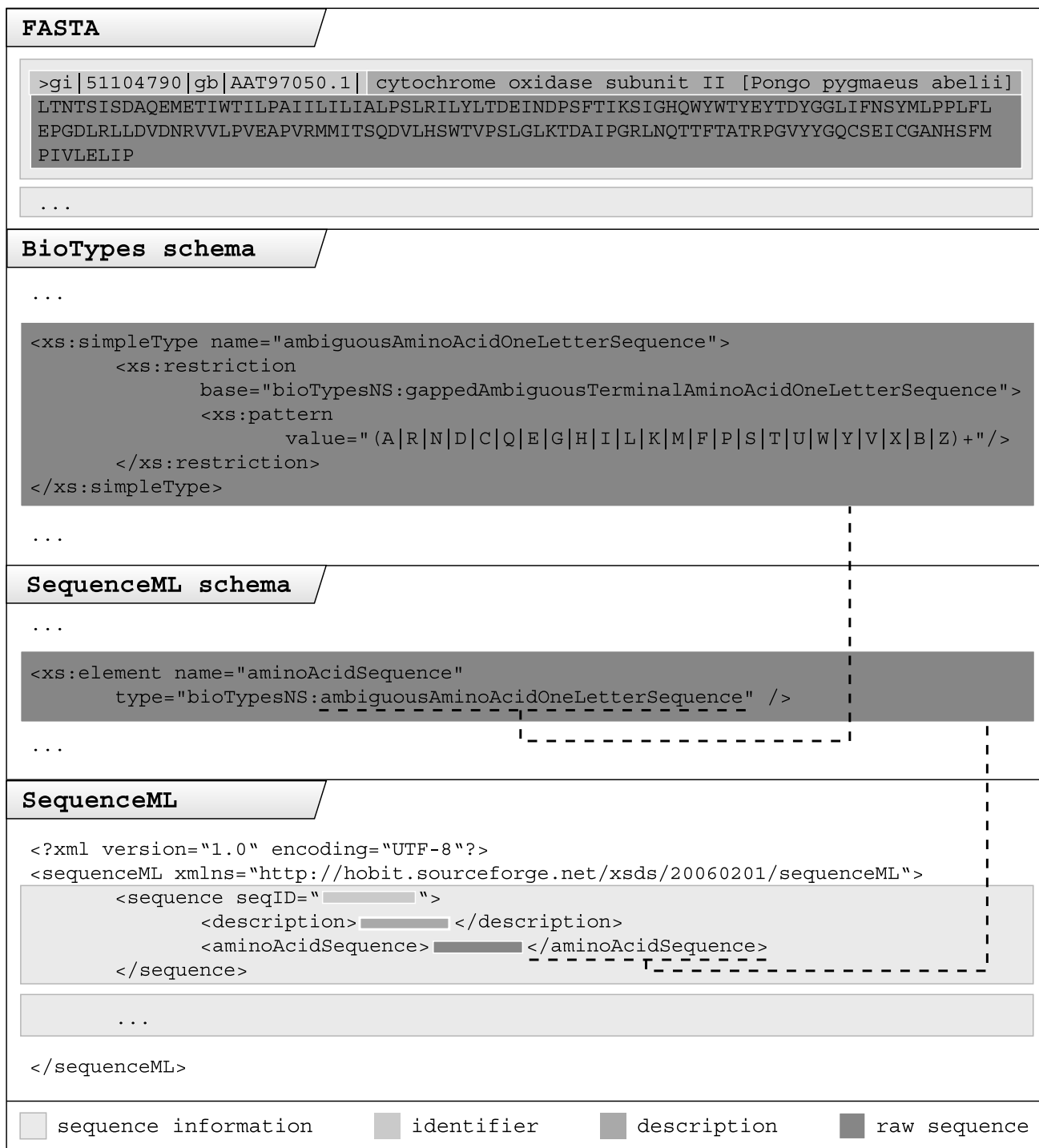
Figure 1 Basic concept of HOBIT XML schemas. The basic concept of HOBIT XML schemas is explained step by step using SequenceML as an example. First an amino acid sequence with id and description in the well known FASTA format is converted to SequenceML. The color coding highlights the transformed content. In SequenceML it is possible to differentiate between various sequence types (in this case an amino acid sequence), defined by the SequenceML schema. The SequenceML schema derives its basic type information from BioTypes.
