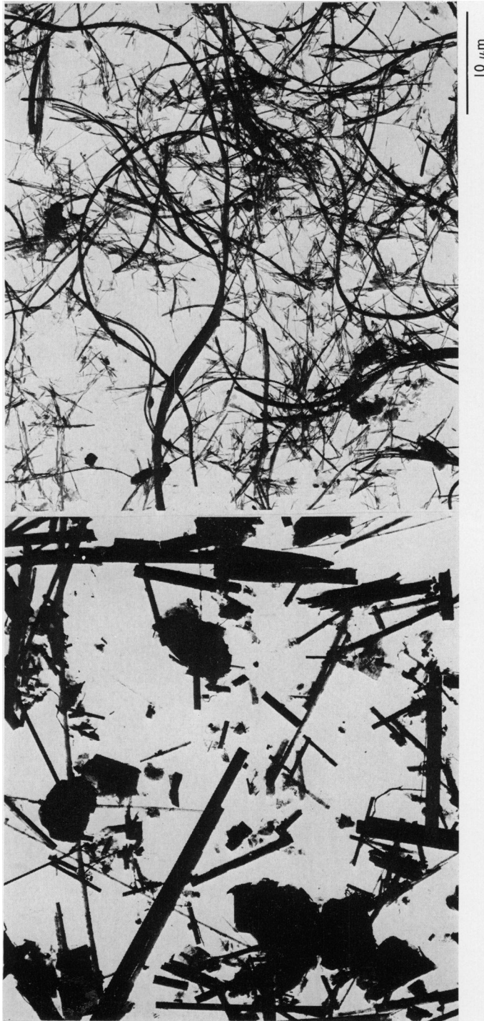
FIG. 5.—Electronmicrograph of UICC anthophyllite ( \times 1875 ).
