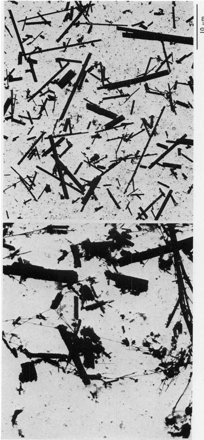
FIG. 3.—Electronmicrograph of brucite ( \times 1875 ).
