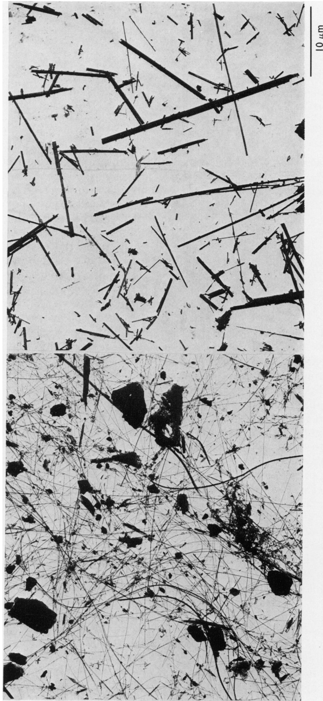
FIG. 1.—Electronmicrograph of SFA chrysotile ( \times 1875 ).
