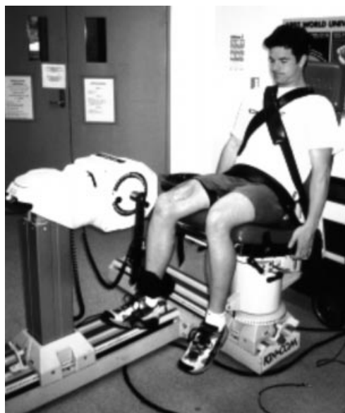
Figure 1 Equipment and subject position for assessment of isometric knee extension and muscle activation. Straps around the chest and waist secure the subject to minimize movement.
