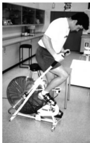
Figure 4 The wind-braked cycle ergometer used in this study allows the measurement of maximal power. The subjects's feet were securely fastened with tape and toe straps to ensure feet were not pulled out of the pedals during the test.
