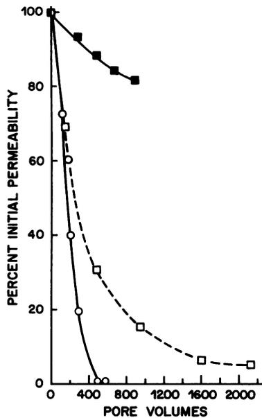
FIG. 1. The different permeability reduction profiles of fused glass bead cores injected with vegetative or starved *K. pneumoniae* cells. Symbols: ○, vegetative culture; □, cell suspension starved in PBS for 2 weeks; ■, cell suspension starved in PBS for 4 weeks.
