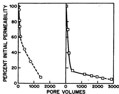
FIG. 6. The permeability reduction profiles of cores injected with bacterial cells (solid line) followed by nutrient stimulation with a [<sup>14</sup>C]acetic acid solution (dotted line). Symbols: ○, vegetative culture; □, cell suspension starved in PBS for 2 weeks.
