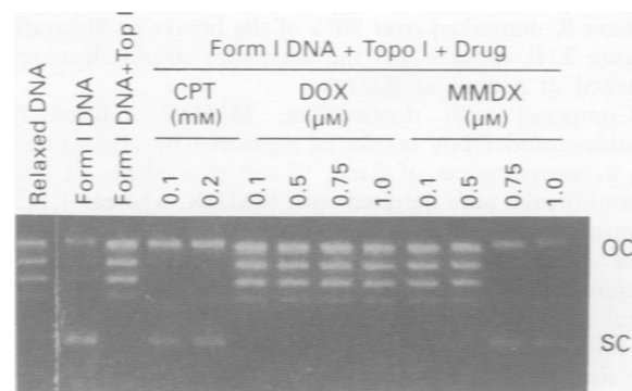
Figure 6 Induction of topoisomerase I-mediated cleavage of a form I DNA (a supercoiled pHOT plasmid) by camptothecin (CPT), doxorubicin (DOX) and methoxymorpholinyl doxorubicin (MMDX). Top I, topoisomerase I; OC, open circular DNA; SC, supercoiled DNA.
