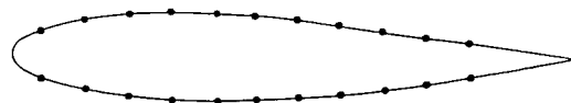
FIG. 4. A comparison of Cayley's sketch of the cross-section of a trout with a modern low-drag airfoil section. Dots indicate trout (adapted from figure 4 in ref. 1).
